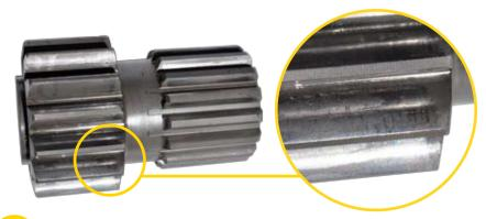
This gear, serviced as per the owners manual shows very little wear, no more than bedin wear after 10 years of simulated augering.
