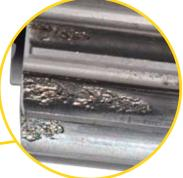
The same drive, submitted to the same work load over 10 years but the oil was only changed once after 5 years. While the drive unit showed no decrease in performance the gear shows visible wear which in time will deteriorate further eventually leading to total failure.
